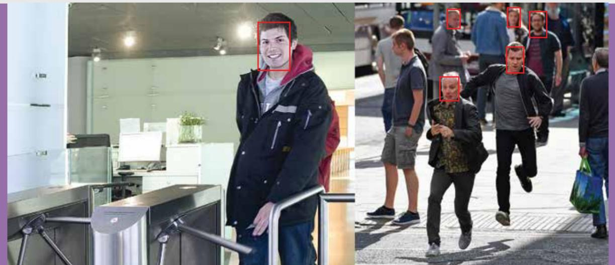
The face recognition module in VideoNet PSIM is a complete element of the access control and management system. Access to the object can be organized in the identification or verification mode.
