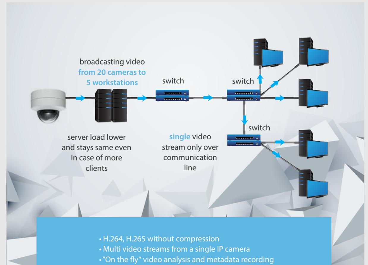
Multicast broadcasting allows to save bandwidth and minimize load on network devices by reducing number of video streams. No video stream
