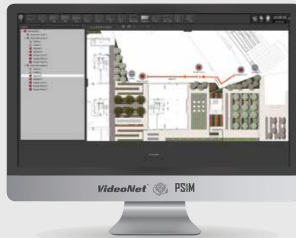
For effective system management, you can locate all perimeter security devices on the graphical plan as they are actually located on your site. You can manage perimeter protection devices using graphical plan window: arm and disarm perimeter segments and perimeter sensors, receive status data from perimeter devices.
